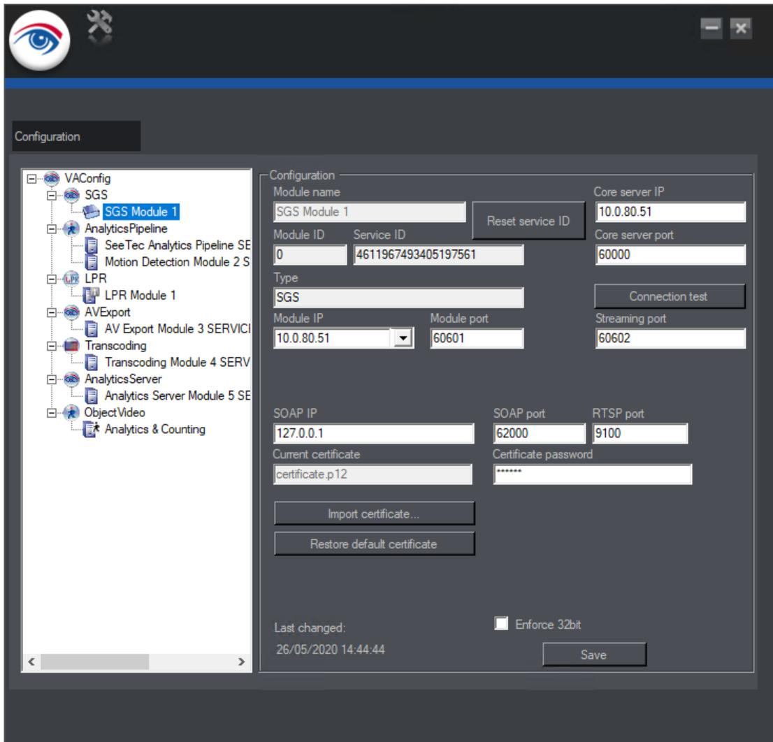
**Fig. 284: Adding a Gateway Service module**
