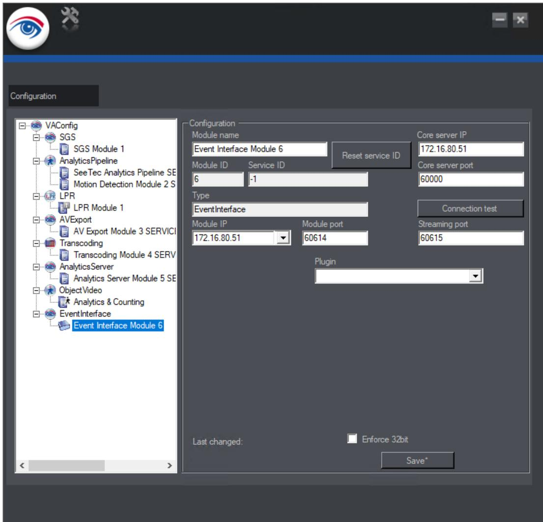
**Fig. 289: Adding an Event Interface Module (SEI)**
