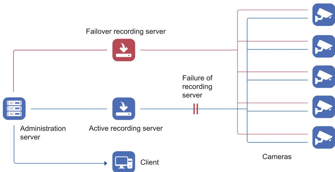
Fig. 5: Fail-safe security via failover concept
