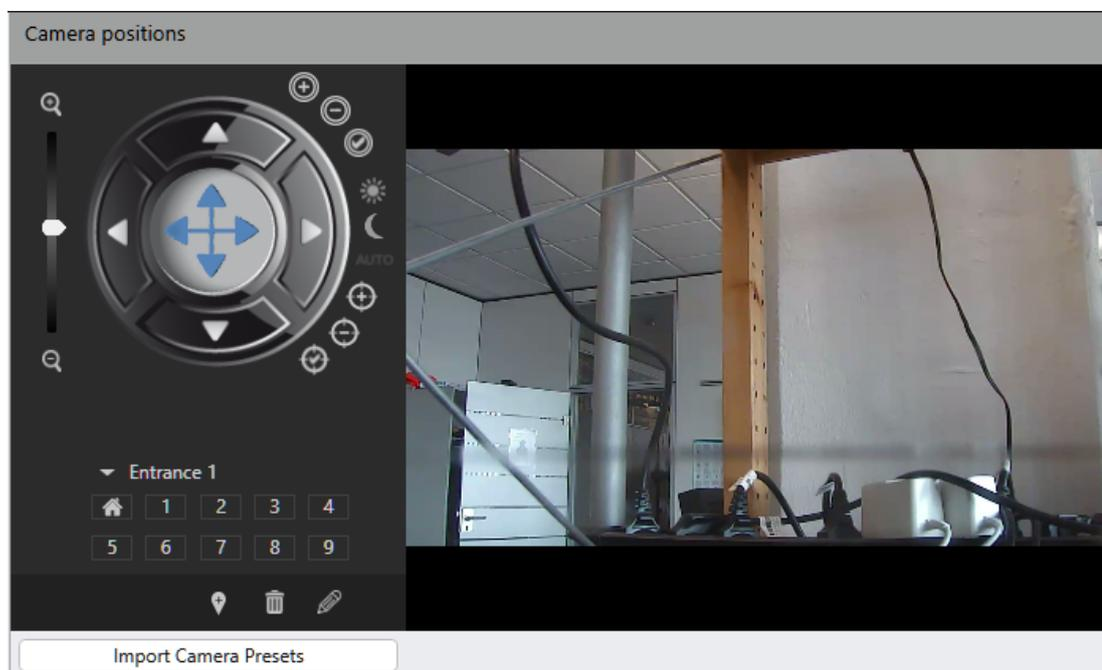
**Fig. 131: Camera positions / digital presets**
