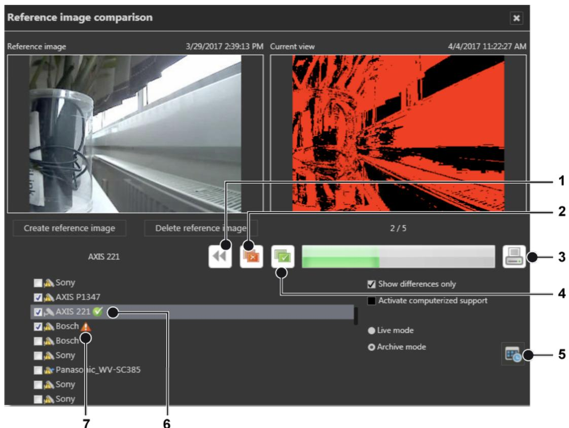
**Fig. 52: Manual reference image comparison**
